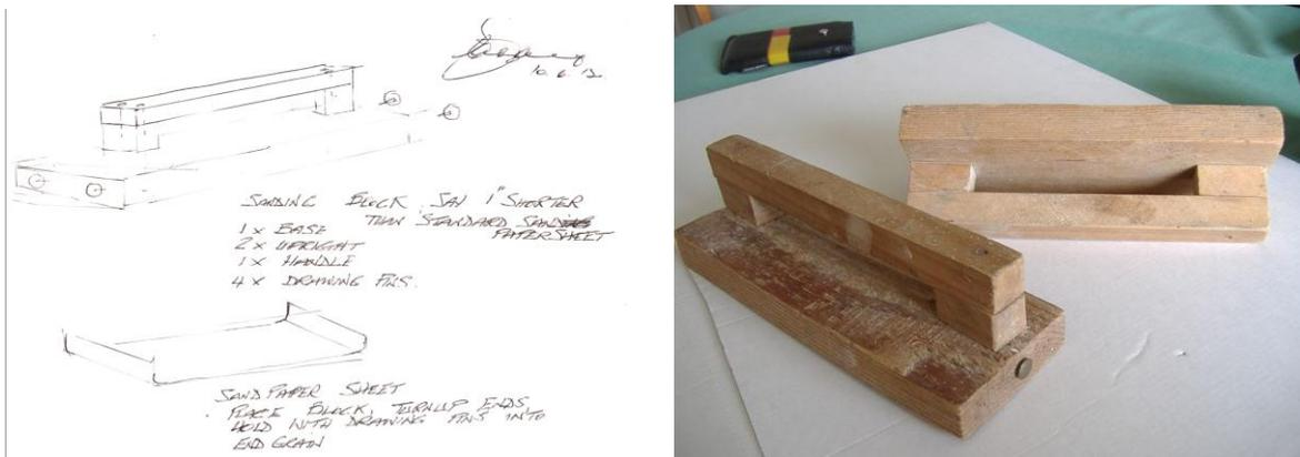
This size works well for smoothing larger surfaces such as a timber slice or table top. It could be adapted for daiza work simply by reducing the measurements.
